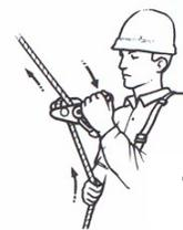
**NOTE:** In order to carry out a rescue, the rescuer requires a harness with a front point of attachment for locating the GRIGRI. If the anchor point for the "GOTCHA™" is such that the casualty must be lowered, then the rope length in the kit must be four times the distance from the anchorage to the point of safety.
